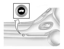
The remote trunk release button is on the driver door.
